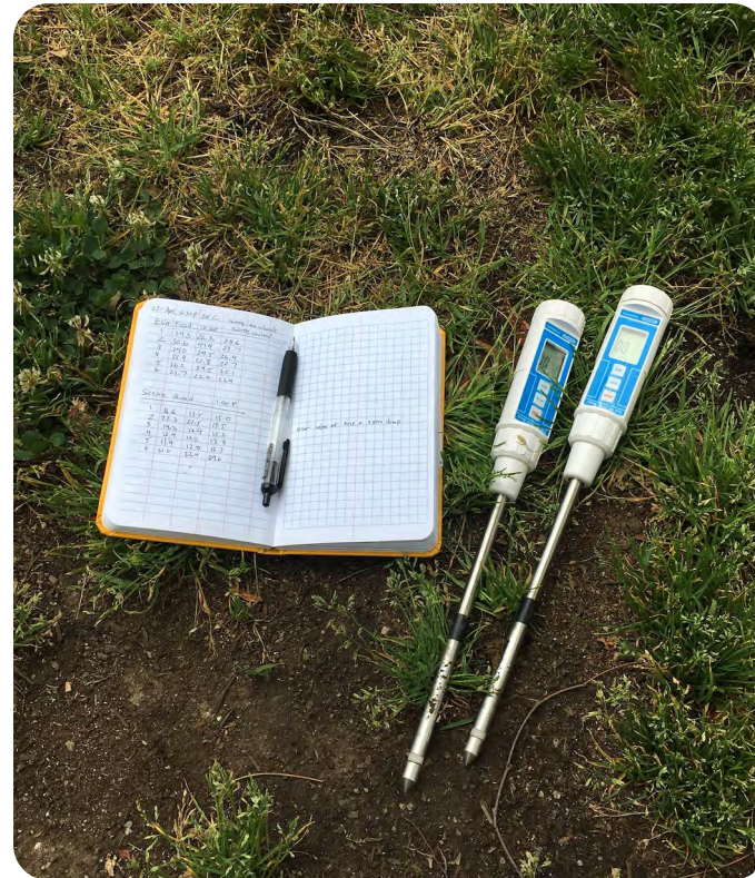
Figure 4. DSMM500 Precision Digital Soil Moisture Meters with Probes used to sample soil moisture content.
