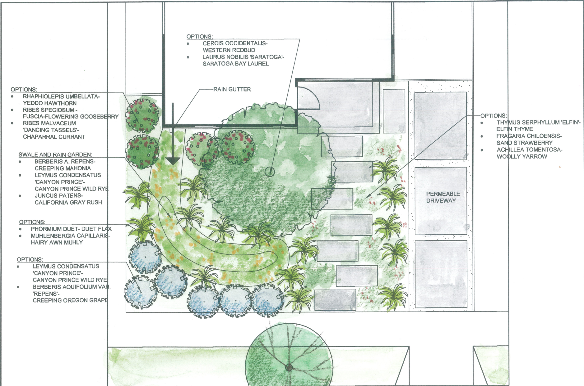
PLAN VIEW FRONT YARD RAIN GARDEN SHADY EXPOSURE
